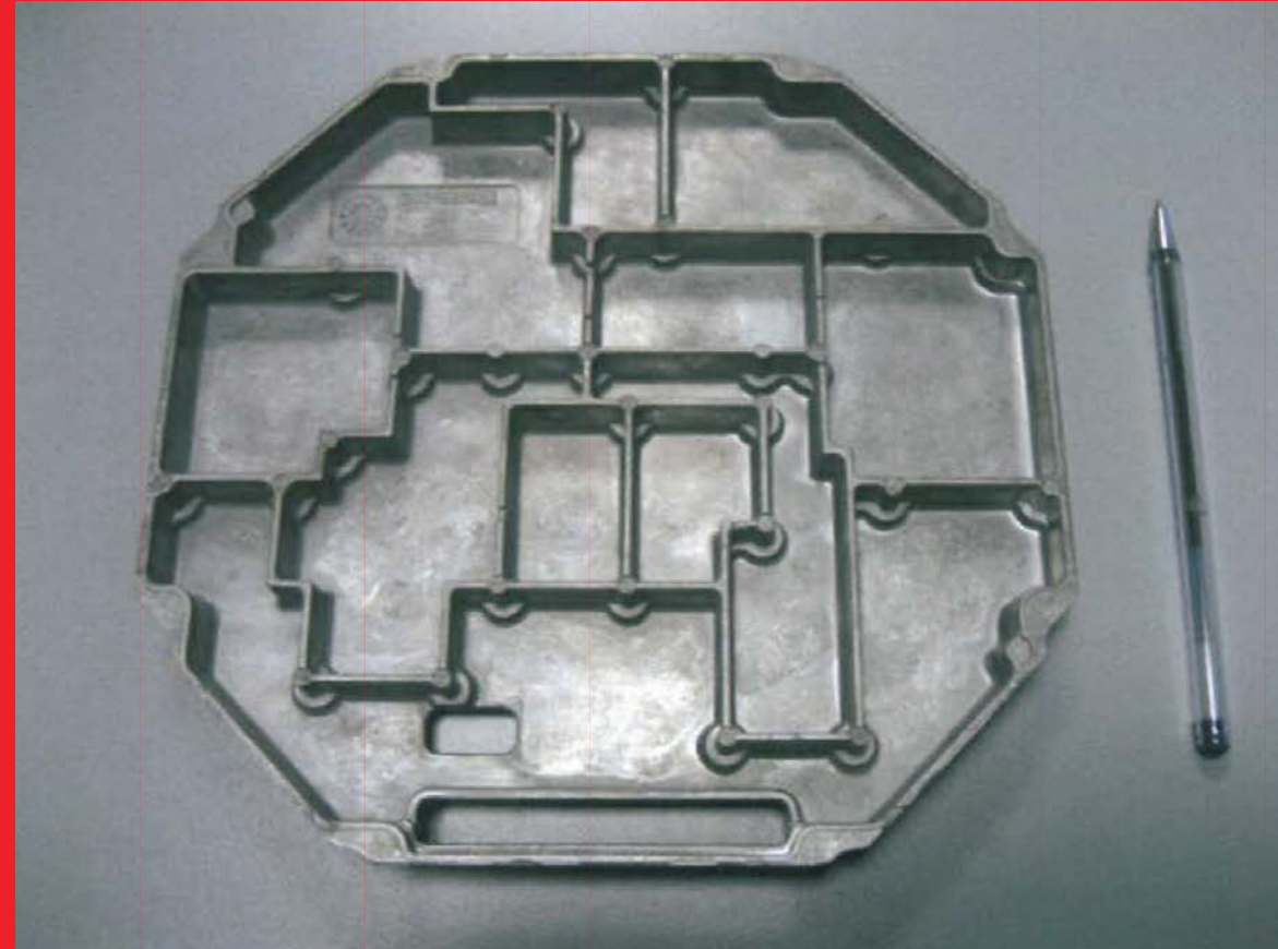
Die Casting of Components Covering the Cutting Blade in a Lawn Mower. Dies were made with Toolox 44.
