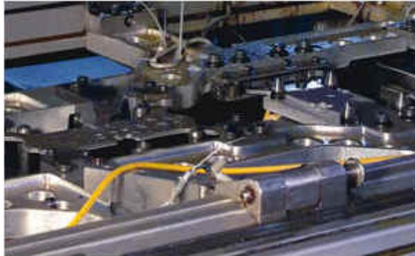
As one of Omni's presses forms the heavy-duty door hinges, a transfer mechanism advances the workpiece to the next station in the die. Because Phyge's FortiPhy™ UltraEndurance™ coating on the four forming inserts inhibits galling and metal pickup, the four inserts last for nearly 200,000 hits, which is approximately 43 percent longer than a CVD TIC coating would last on the same tool steel.
