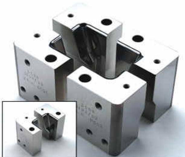
Omni had this set of four forming inserts stripped, polished, and recoated with Phygen’s coating. The coating has the adhesion and wear resistance of CVD processes, but because it is applied at a relatively low temperature, it does not distort the tooling. This characteristic lends itself to recoating the tooling over and over again.
