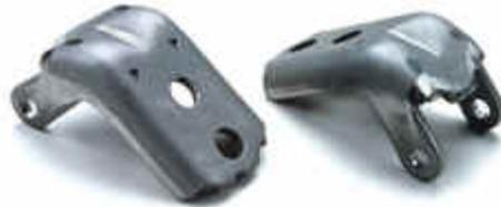
Producing these heavy-duty door hinges is 10 times more economical since Omni switched both the substrate and coating on the inserts that form them inside the stamping die.
