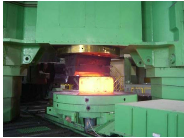
Photo 2. SUS304N2 disc under forging
