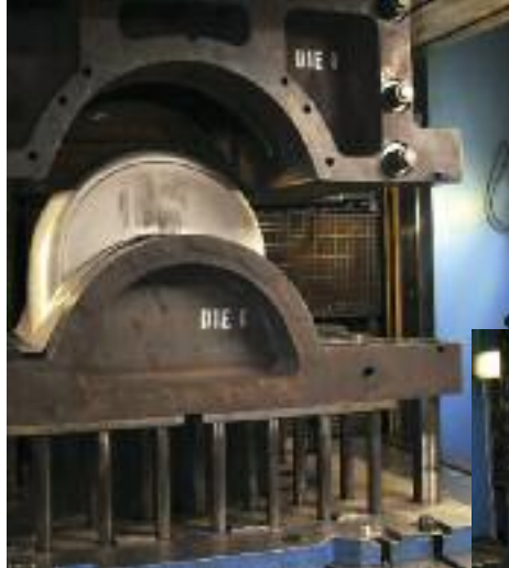
Type 304L stainless-steel blanks, 20 gauge, are deep drawn in an 850-ton AP&T hydraulic press, then laser-trimmed in a five-axis Prima cutting machine before undergoing a final restrike in a 1000-ton hydraulic press.
