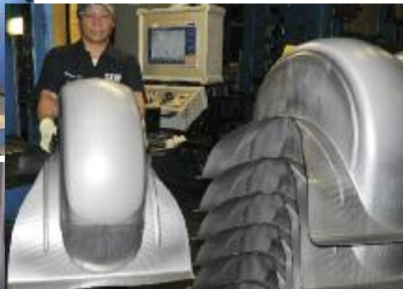
Type 304L stainless-steel blanks, 20 gauge, are deep drawn in an 850-ton AP&T hydraulic press, then laser-trimmed in a five-axis Prima cutting machine before undergoing a final restrike in a 1000-ton hydraulic press.
